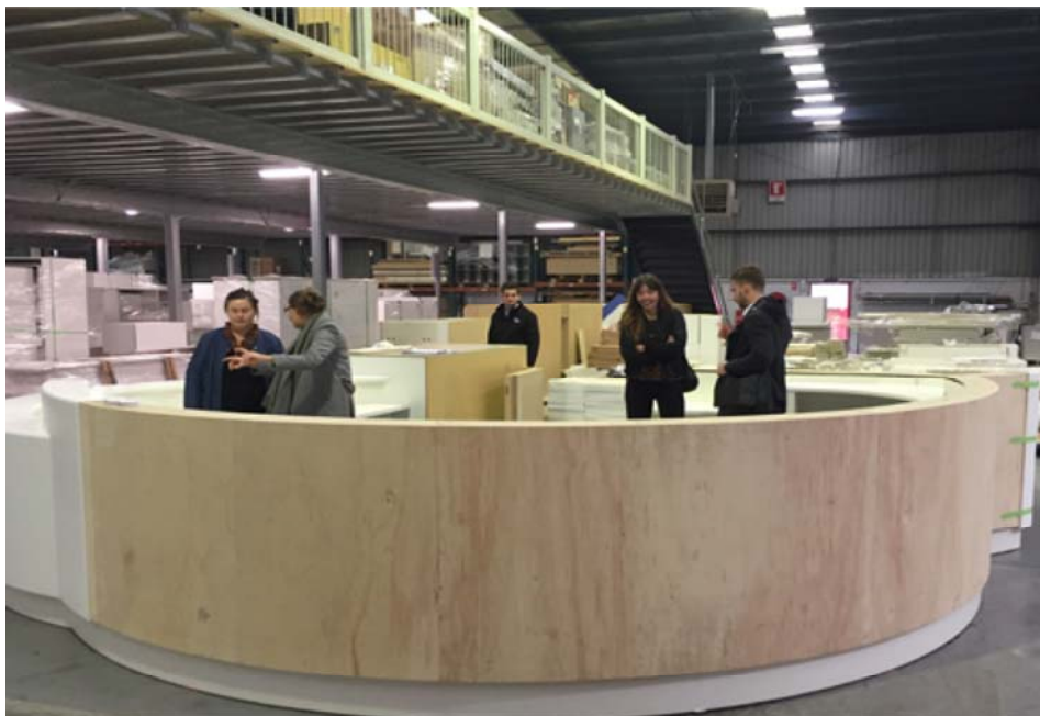
The photo above is of the architects visiting the factory that is making the joinery for JKWCH. They are standing in the reception desk under construction for the ground floor.
